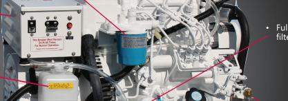
Full flow, spin-on oil filter with bypass
